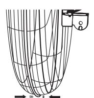
Step 6: Secure the assembly of front guard and rear guard by tightening a screw and nut at the bottom position.
