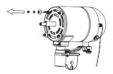
Step 2: Remove four sets of hexagonal nuts,
