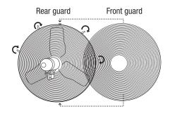
Step 5: Assemble front guard to rear guard by fixing both guards together with clips.
