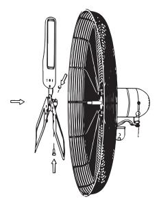
Step 4: Assemble fan blade onto motor shaft by tightening the two screws which are located on fan blade. Make sure screw are tightly secured.
