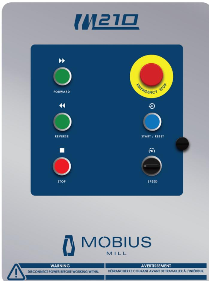
**E-STOP** - Emergency stop button – stops all moving parts on the device.
