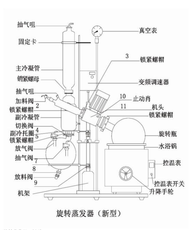
旋转蒸发器(新型)rotary evaporator(new type) 抽气阻 air exhaust mouth 固定卡 fixing clip 主冷凝管 main condenser pipe 销紧螺母 jam nut 加料阀 charging valve 锁紧螺帽 lock nut 副冷凝管 vice condenser pipe
