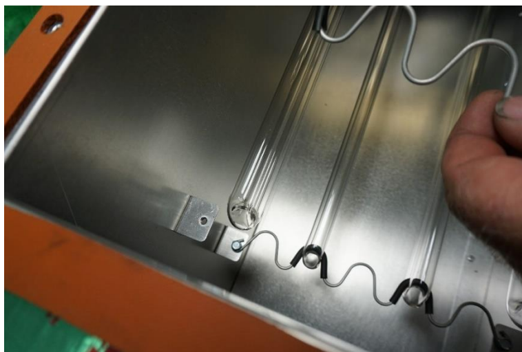
Figure 5: Remove bulb support wires and place aside
