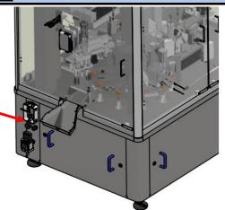
The connection is made with a passthrough connector located between the electrical power and the compressed air solenoid valve.
