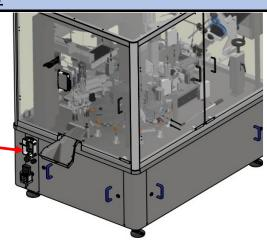
Using a passthrough connector, the cable goes through the disconnect box for wiring to be done inside.
