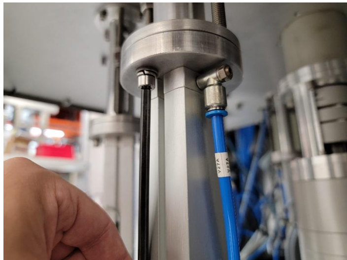
Figure 4.7: Unscrewing a cylinder underneath the machine
