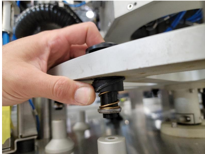
Figure 4.2: Removal of the O-Ring with the fingers
