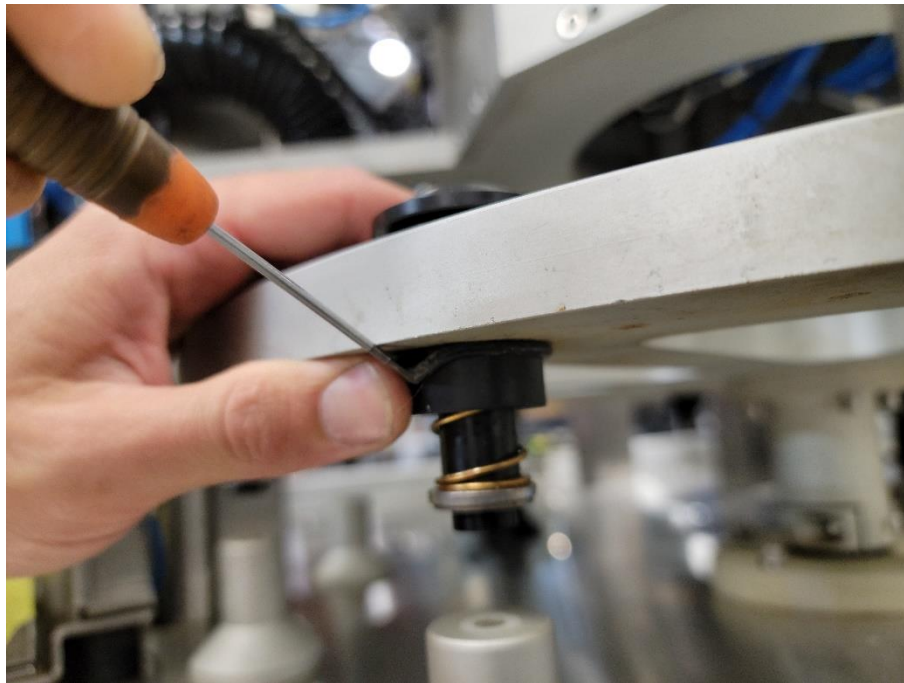
Figure 4.1: First step to remove the O-Ring of the cone holders
