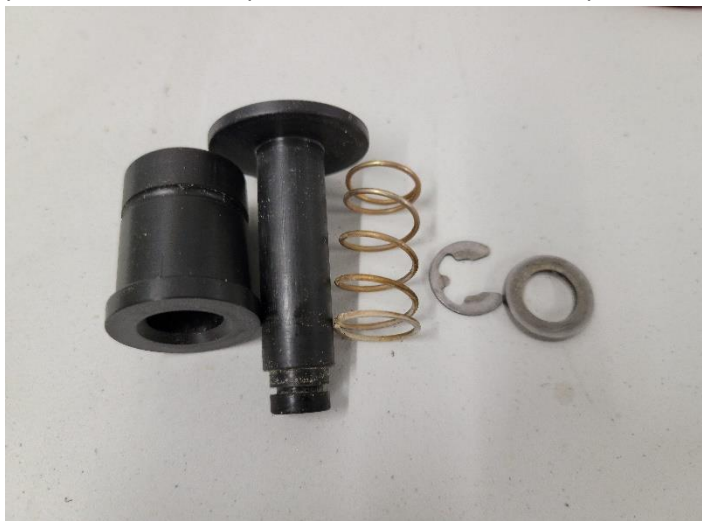
Figure 4.4: Components to clean when the holder is disassembled
