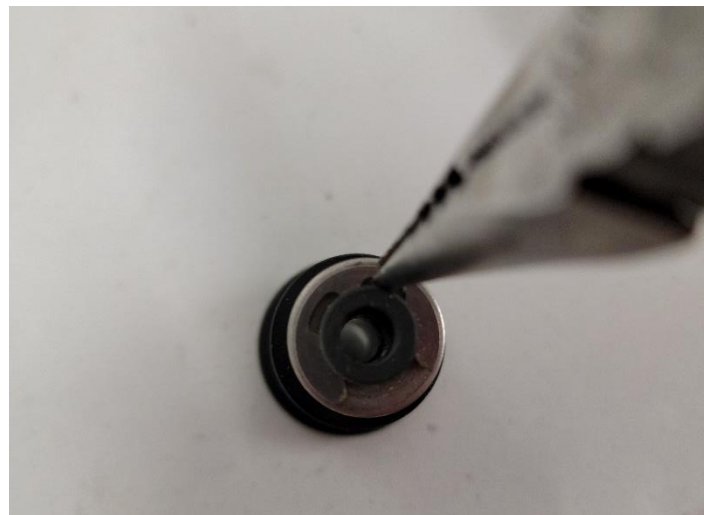
Figure 4.3: Position of the longnose to remove the retaining ring
