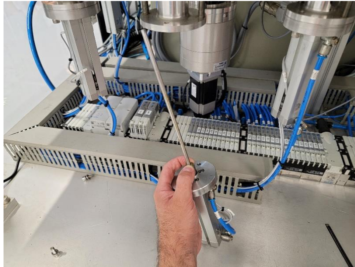
Figure 4.8: Angle required to remove the cylinder
