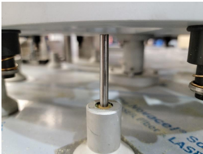
Figure 4.5: Position of push rod when it's ready to be cleaned
