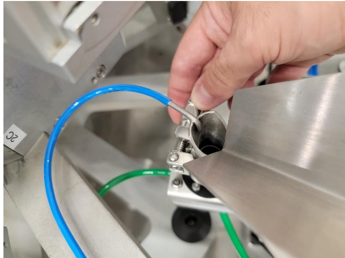
Figure 4.18: Untighten the bolt to remove the nozzle
