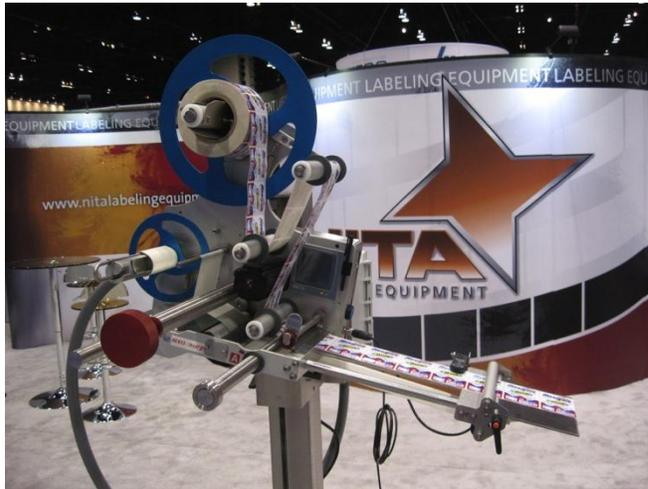
A good adjustment is when the exit of the label is at a 15 to 20 degree angle against the surface of application.
