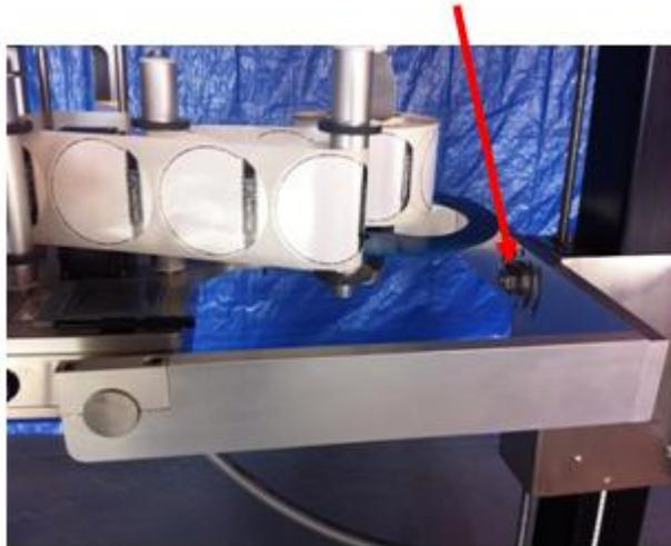
To adjust the angle or rotation of the labeller head (when equipped with the holder), slightly loosen one of the two Allen screws on either side of the labeler's bracket, position it to the required angle and re-fasten the screws (be careful!).
