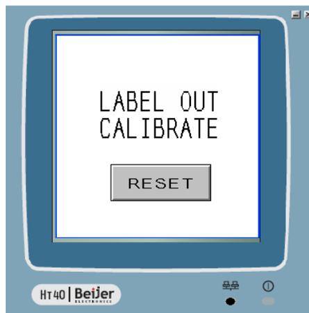
To reactivate the system, after solving the problem, simply press the Reset key. It will lead you to the screen of the faulty labeling head and will stop the audible alarm. You will have to reposition the web (or tend to empty roll) and restart the system.
