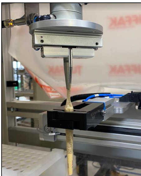
Figure 16: Station #2 showing the Pick and Place Arm and Stationary Grippers (Twist).
