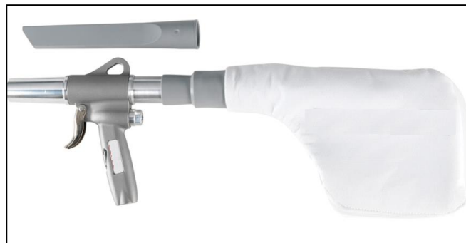
Figure 47: Air blow gun and venturi vacuum
