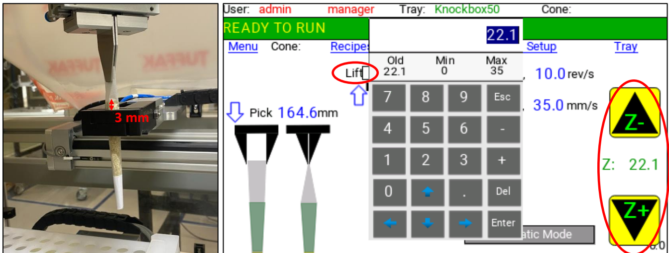
Figure 42: Cone Lift position setup
