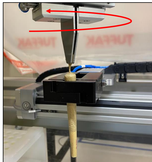
Figure 16: Station #2 showing the Pick and Place Arm and Stationary Grippers (Twist).
