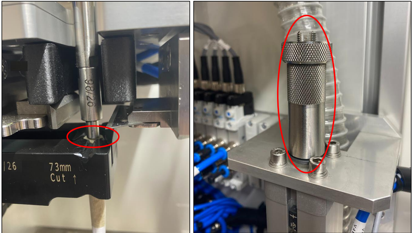
Figure 46: Flat Top rod depth setup
