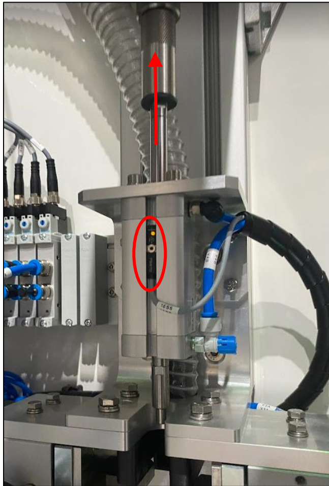
Figure 56: Top Crusher Home position
